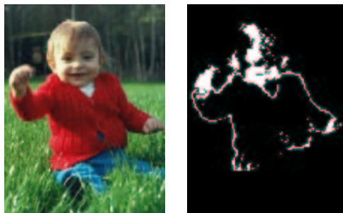
Figure 1: Result of the color filter on a color image. White pixels correspond to skin color
